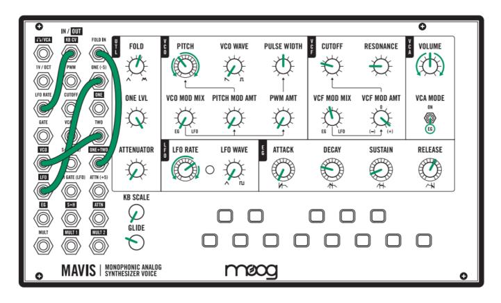
• Tune the VCO and LFO to a unison via the LFO RATE and PITCH knobs.
