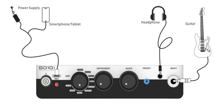
**Notes:** When the device is connected to a headphone, the speaker will be muted.
