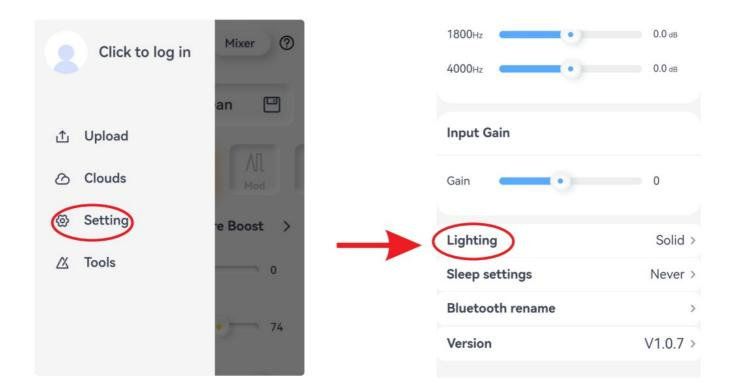
To avoid the power consumption caused by not being powered Off when the device is idle, we designed the sleep mode for the SD10i.
