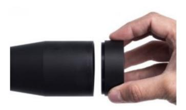
This scope includes a honeycomb sunshade. It will prevent light from reflecting off your glass, reducing outward glare and help conceal your position. To attach, unscrew and remove the thread protector on the Accessory Attachment ring and then screw into the now exposed threads.
