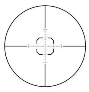
The G2-FFPS1624 Scope is equipped with a MOA-X1 reticle. Features 2 MOA hash marks spacing on windage and elevation posts, extends by 20 MOA in each direction. 1 MOA = 1 inch at 100 yards.
