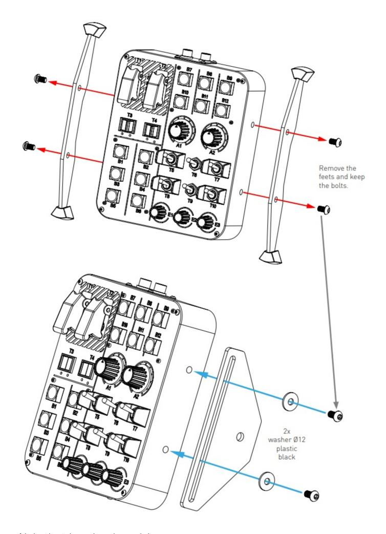
A locknut has to be rough-running on a bolt. Therefore you need to use a wrench and a hex key to tighten it. Hold up the M8x18 bolt with the hex key while
