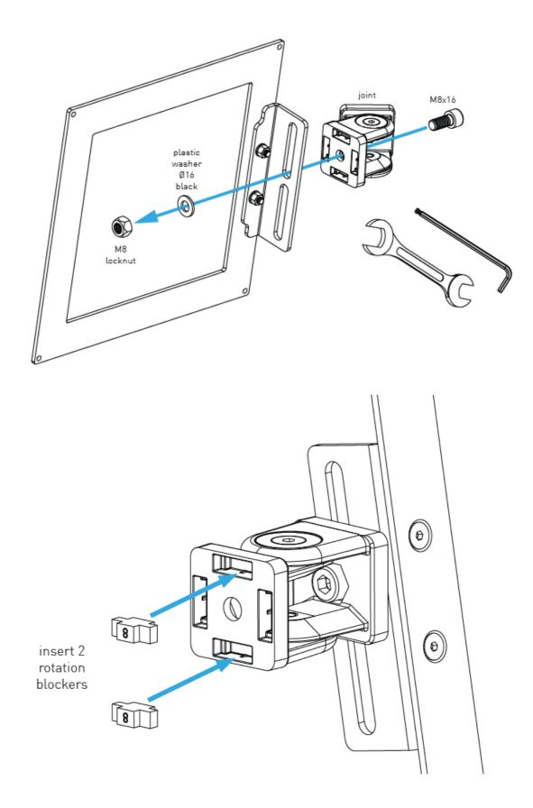
• Assemble the Apache MPD same way as shown for center assembly on page 7-8.
