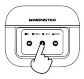
Provide 16 levels of volume adjustment function, click the button to increase/decrease volume (Volume increase or decrease can only be operated by opening the cover of the charging compartment or removing the headset)
