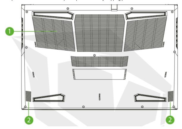
The thermal vents are designed to cool the internal components and avoid overheating.
