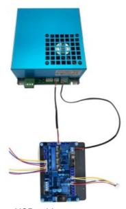
• Step 3: Connect the machine with PC via a USB cable.
