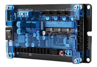
This GRBL controller is developed for Monport 40w CO2 laser engraver & cutter and other 40w machines which can engrave and cut glass, leather, plastic, wood, etc. Its firmware and ports can also be used to control similar engravers from other manufacturers and some CNC machines. It can be taken as the replacement of Nano controller.
