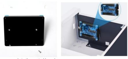
• Step 2: Connect power supply to the control board.
