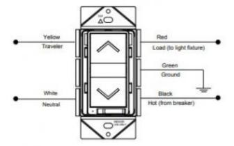
**Important Note:** Despite the presence of the Traveler line, this dimmer switch does not support the 3-way switch function. Do not use the traveler line.
