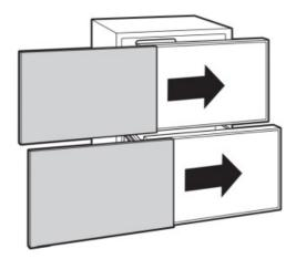
• Reinstall the side trims using the trim screws removed earlier.
