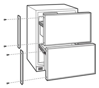
Custom handles of your choice, supplied by your cabinet maker, must be installed onto the overlay panels before
