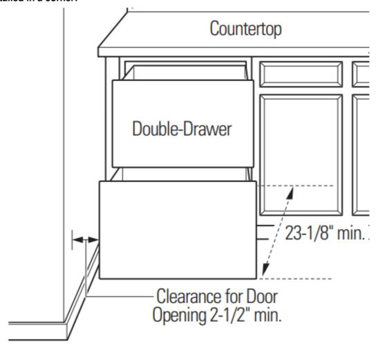
Allow 2-1/2" min. clearance between Double-Drawer and adjacent cabinet, wall, or other appliances. Allow 22" min. clearance from the front for drawer opening.
