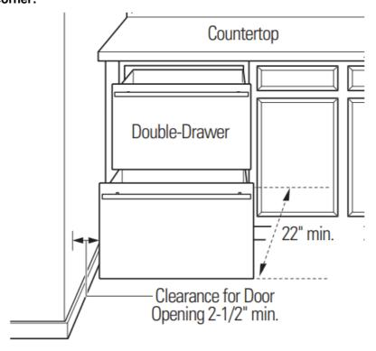
Allow 2-1/2" min. clearance between Double-Drawer and adjacent cabinet, wall, or other appliances. Allow 23-1/8" min. clearance from the front for drawer opening.
