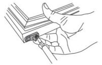
• Remove the black screw post from the bottom of the door using a flat head screwdriver. Keep the screw post.
