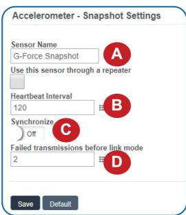
**Note**: Be sure to select the Save button anytime you make a change to any of the sensor parameters. All changes made to the sensor settings will be downloaded to the sensor on the next sensor heartbeat (check-in). Once a change has been made and saved, you will not be able to edit that sensor's configuration again until it has downloaded the new setting.
