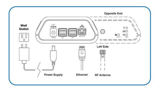
1. Power up the Advanced Edge Gateway by first plugging in the power supply and connecting the Ethernet Cable. It may take up to two minutes for the indicator LEDs to show activity.
