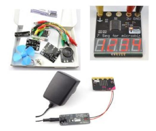
From left to right: Electronics Starter Kit for micro: bit, Power for micro: bit (AC adapter not included), and 7 Segment for micro: bit.
