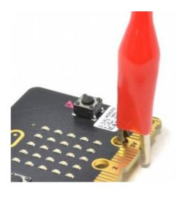
Connecting the alligator clips like this prevents any accidental connections between the large connectors with the holes in and the much smaller connectors (gold lines in the photo above)
