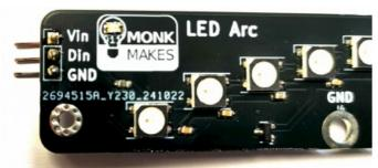
If you want to mount the LED Arc in an enclosure, and the LEDs are going to be against a front panel of some sort, then it's best to push the short end of the right-angle header pins through from the bottom of the LED Arc and solder on the top (as shown above) – as this will make it easier to attach leads.
