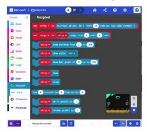
The most important block, without which nothing will be displayed, is the first one in the example code below.
