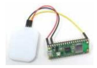
Or, you can put your Pico in breadboard and connect it with female-to-male jumper wires. Using Breadboard for Pico (<a href="https://www.monkmakes.com/pico\_bb">https://www.monkmakes.com/pico\_bb</a>) will make it very much easier to identify which pin of the Pico is which.
