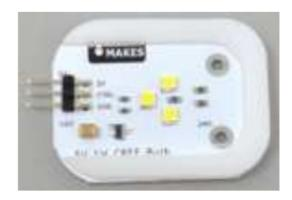
Then press the backwards-C shaped diffuser piece onto the PCB taking care not to get any glue on your fingers. Leave it to set for a couple of minutes before carrying out the next step.
