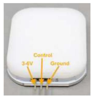
As well as turning the illuminata on and off, you can also control its brightness by connecting the Control pin to a PWM (Pulse Width Modulation) output pin.
