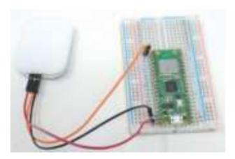
or, you can just mount the Illuminata end-on on the breadboard and use male-to-male jumper wires to make the connection.
