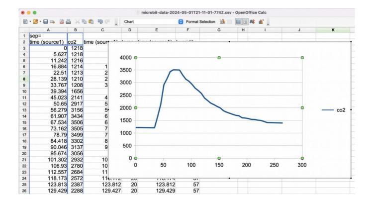
Because the three readings are actually logged at slightly different times, there will be a separate time column, in the CSV file, for each reading type. When creating a chart, just pick one of the time columns for the x-axis – it doesn't matter which. This project uses the serial write value block that you will find in the Serial category of blocks. This sends the reading over the USB connection to the makecode editor running in your computer's browser.
