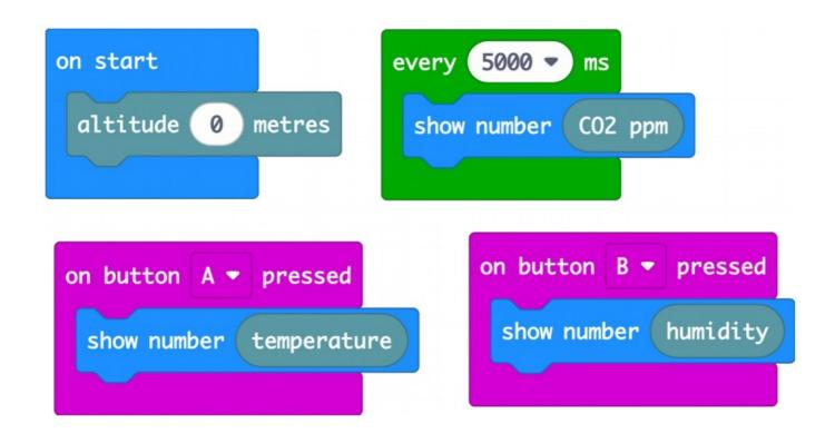
Install this program onto your micro:bit in the same way as you did in experiment 1, by using the code link at the top of this page. When you press button A, the temperature in degrees C will be displayed once the current CO2 reading has finished displaying. Button B displays the relative humidity (how much moisture is in the air).
