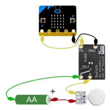
This project uses the micro:bit's built-in light sensor to measure the level of light and when it falls below a certain level, it activates the Switch or Relay and turns on the LED lamp. Hold your hand over the micro:bit's display to simulate it going dark. This should cause the LED lamp to turn on.
