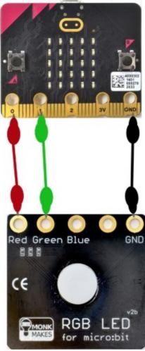
Then connect the RGB LED as shown to the right. Try moving your micro:bit. As soon as you do, you should hear a tune start to play to indicate that the alarm has been triggered and the RGB LED color will change from Green to Red.
