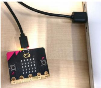
If your micro:bit is new, then its LED display will start displaying messages and showing off various features of the micro:bit. You are going to replace this program currently running on your micro:bit with a new one.
