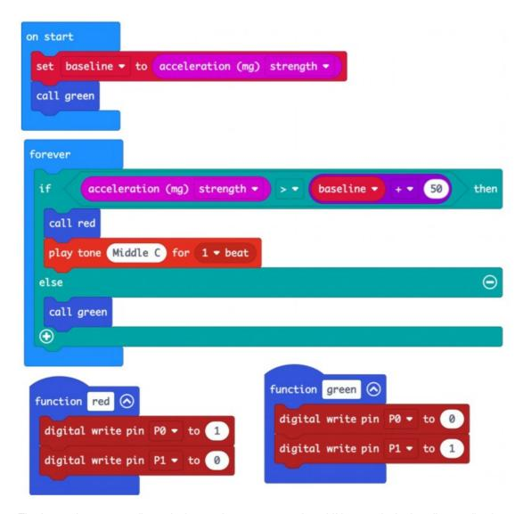
The forever loop repeatedly reads the accelerometer strength and if it exceeds the baseline reading by 50, the alarm is sounded. The functions red and green set the RGB LED color to red or green, by writing a 1 or a 0 to the appropriate pins controlling the RGB LED red and green channels. Try tweaking the number 50 in the if block, to alter how sensitive the alarm is.
