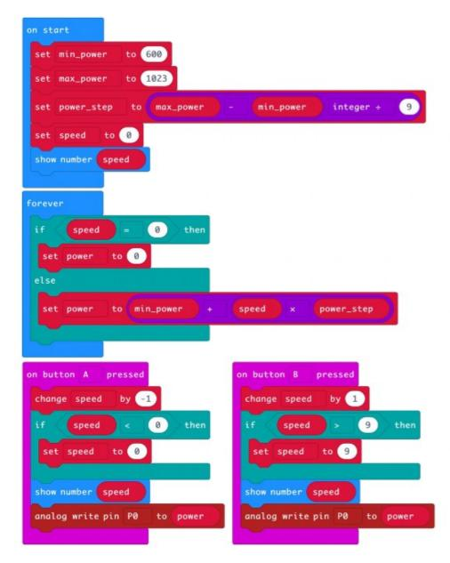
The on button pressed blocks are very similar to each other. The block for button A subtracts 1 from speed while making sure that speed does not fall below zero and then displays the new speed and uses analog write to set the power output of pin 0. The on button pressed for B does the same kind of thing, but adding 1 to speed.
