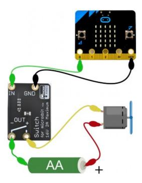
This project uses exactly the same wiring as Project 5, but uses the micro:bit 2's built-in microphone to toggle the motor on and off when a loud noise such as a clap is detected.
