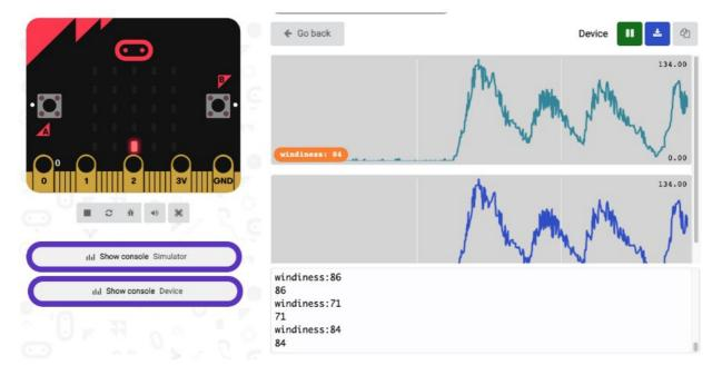
Each set of peeks corresponds to a strong blow onto the fan blade. You could use this to measure the maximum speed to see who can blow the hardest.
