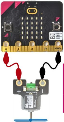
**WARNING:** Flash the program P4 Anenometer onto your micro:bit BEFORE connecting up the motor. Failure to do so could damage your micro:bit. Also make sure that you connect the motor as show, with the motor's + connection to micro:bit pin 0. Also, this project if fine for lung power, but a very high speed of rotation could damage your micro:bit.
