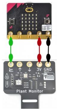
As before, power is supplied by the micro: bit, but this time, micro: Bit pin 0 is used to connect to the analog output of the Plant Monitor.
