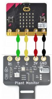
The red and black leads provide power from the micro: bit to the Plant Monitor and the yellow and green leads send serial data to and from the Plant Monitor.
