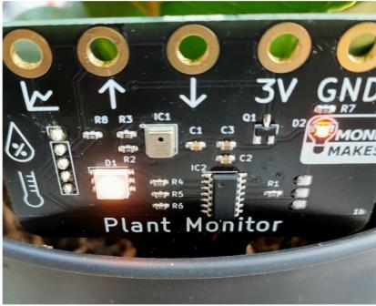
The front side of the prong should be as close to the edge of the pot as possible.
