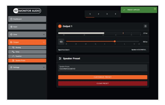
If using one of the Climate Garden loudspeakers, the preset needs to be tweaked slightly because the 100v line option gets reset when loading the preset.
