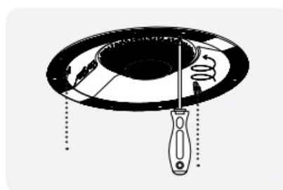
Push speaker into hole and tighten all 3 Tri-Grip Dog Legs
