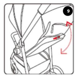
7. USING THE FOOTREST - FIGURE 10: To adjust the footrest, hold the button on both sides for its release.
