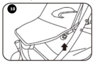
8. **ATTACH AND DETACH THE SAFETY BOARD – FIGURE 11:** Insert both ends of the safety board into the two side holes of the frame. Secure the guard until you hear a click. To remove the guard, press the release button on both sides of the frame and pull at the same time. The safety bumper has the function of pivoting, it can be opened on just one side for easier taking care of a baby or putting it in or taking it out.
