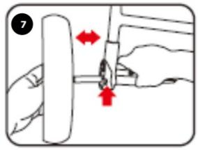
5. **USING THE BRAKE ON THE REAR FRAME**— **FIGURE 8:** To activate the parking device and lock the two rear wheels, press down the pedal on the rear axle (Figure 8). To release the brake, pull up the pedal using your foot.
