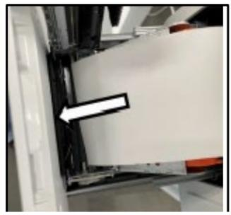
4. Feed the paper through the opening on the printer door.
