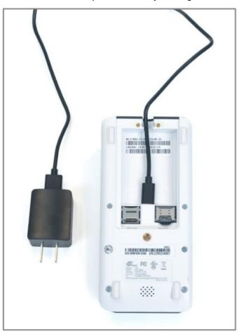
3. Replace the battery plate and screws securely using a screwdriver. Ensure the other end of the cable is securely plugged into the DC adapter.
