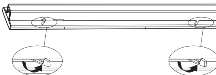
Picture 6 If the fixing lock position is interfered, slide it to right or left to avoid track joint.
