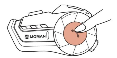
Reject the call: press and hole the Function Key for 3 seconds until you hear the "beep" sound.
