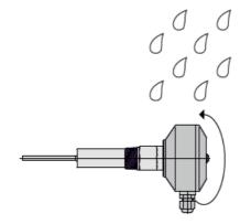
The cable glands must always point downwards to prevent moisture seeping inside the housing. If the housing is not in the correct position after the probe has been firmly screwed into the bin wall, proceed as follows:
