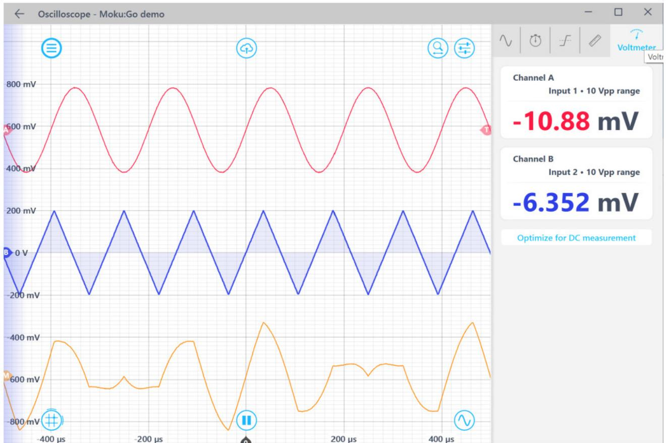
The Optimize for DC measurement button auto-scales each channel's y-axis such that the entire DC signal is viewable in the signal display area for better mean calculations.
