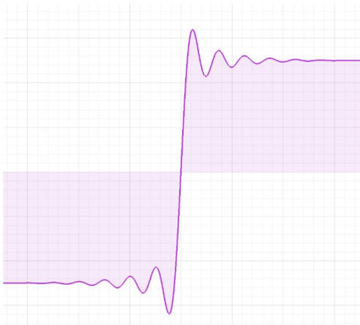
Also called “Sinc” interpolation, this mode preserves the frequency characteristics of the signal. In the time domain, it can appear that there is over- or under-shoot that is not present in the signal.
