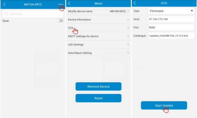
**Note:** The OTA server (Host: 47.104.172.169, port: 8080) in the above picture is just available for your test. If you need, MOKO can provide the lasted firmware upgrade packet, and then you can paste the file to your server to operate OTA.
