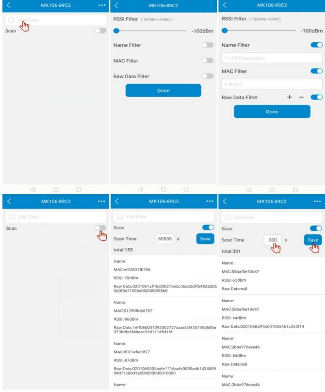
Note: If all filters have been set, device will execute each filter rule as "And" operation.
