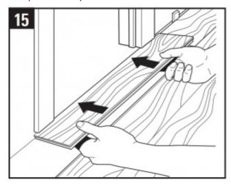
16. Tap the long side joint closemd first. Then tap the end joint closed.
