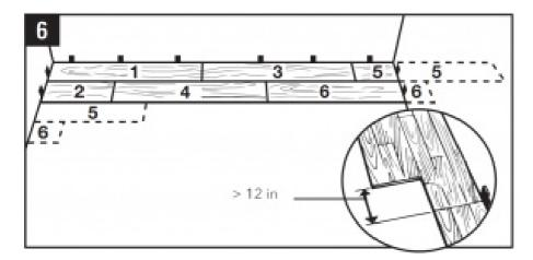
7. At a slight angle, insert the tongue of plank 2 into the groove of plank 1 until the RevWood Contract edges meet, and then rotate down until the joints lock.
