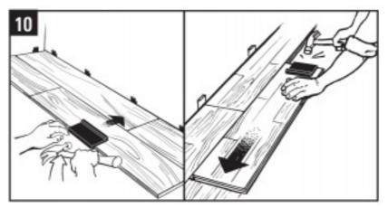
11. Ensure there will be a 3/8" gap (after the joint is closed) to the wall and all vertical objects for expansion.
