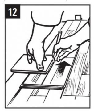
13. For the last row, install the long side tongue into the groove with the end joint aligned. Using a pull bar and hammer, work evenly along the length of the plank and lightly tap the joint closed.
