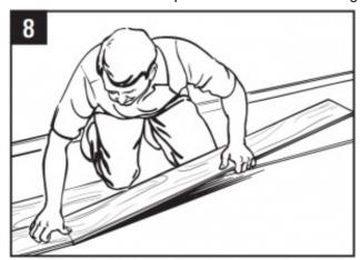
9. Raise the outside edge of the plank upward approximately 1". Maintain this angle as you push the plank in until the RevWood Contract edges meet. Rotate downward on the plank until the joint locks. Repeat these steps to complete the installation.
