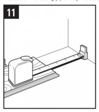
12. For the last row, align the plank to be used on top of the second to last row. Using a full width plank as a
