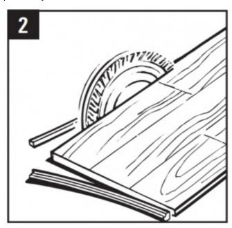
3. For uneven walls, trace contour on tongue side of plank and cut.
