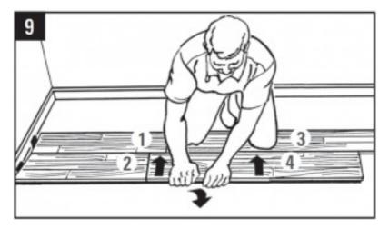
Installation Tip: Place a carton of planks across the end of the row being installed to keep installed planks in place during installation.
