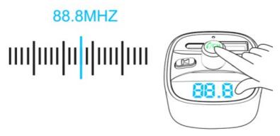
3. Tune the device to the same channel as the car radio.
