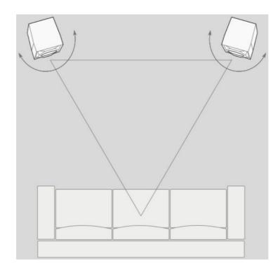
Imaging is often overlooked when listening of stereo speakers. If correctly spaced and arranged with an optimal toe-in angle, these speakers can create a large involving soundstage while retaining focused imaging.
