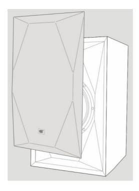
The grilles magnetically attach to the speakers. To affix, simply hold a grille by its edges and hold it up next to the front baffle. It will automatically pull itself to the baffle and self-locate. To remove it, hold the edges and pull it away from the baffle.
