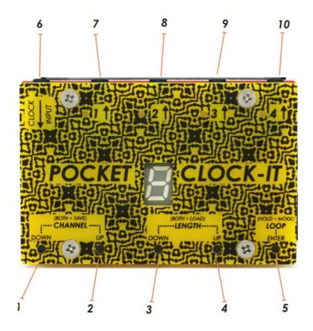
HOW TO SWITCH MODES: Hold LOOP / ENTER button to switch modes. When a lowercase "r" is displayed, POCKET CLOCK-IT is in random mode. When an upper case "C" is displayed, POCKET CLOCK-IT is in clock divider mode.
