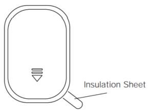
Remove the insulation sheet to power on the sensor.
