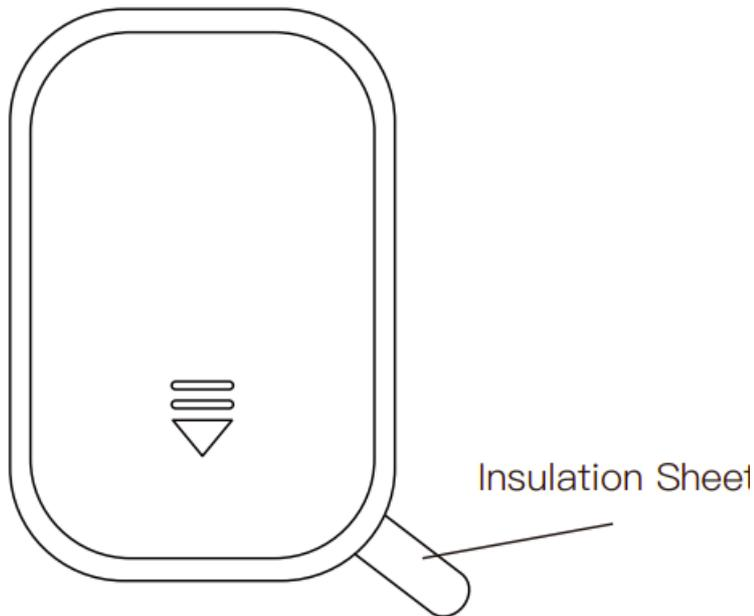
Remove insulation sheet to power on the sensor.
