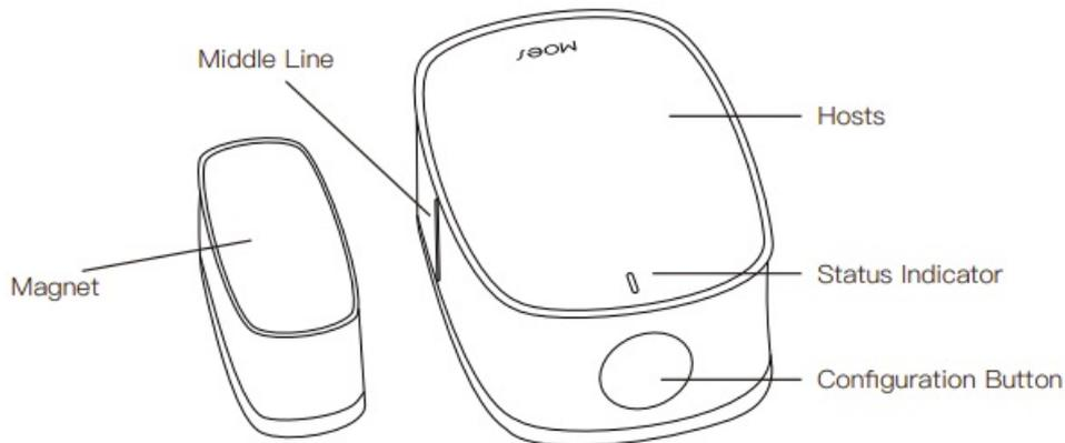
Make sure the side of the magnet with marked line is aligned to the side of the hosts marked with the Middle line.
