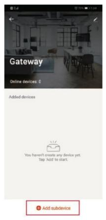
4. Click on "Add subdevice" and wait for the device's LED to blink to initiate the device search.
