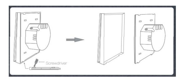
• Mount the switch with the provided screws and snap the wall plate on it.
