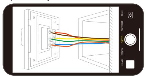
• Follow the wiring diagram to connect the switch wires to the wires in the wall box with the wire conductors.
