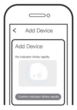
Make sure your smart phone and WiFi+RF switch module are under the same WiFi network at2.4GHz connection. Confirm when the light blinks rapidly (twice a second).
