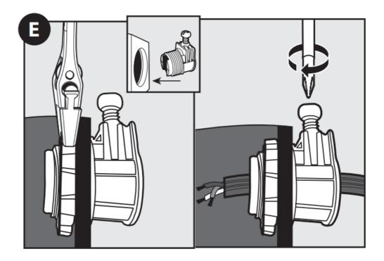
Insert cable connector (not included) into the access hole and secure by tightening the nut. From wall, insert power supply cable through the connector and tighten connector.
