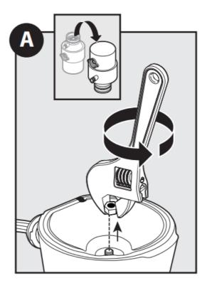
With power supply turned off, remove metal plate on the bottom of the disposal.
