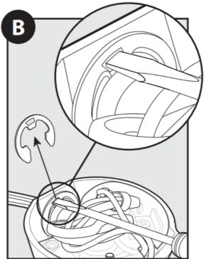
Remove clip with needle nose pliers or flathead screwdriver from the strain relief piece of the cord, and remove cord.
