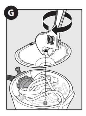
Push wires into the disposal and replace the metal bottom plate (do not displace plastic shield with label).
