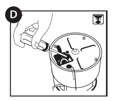
Turn off power at circuit breaker or fuse box. When the old disposal is removed from sink flange, disconnect any hardwired connections or unplug unit. Disclaimer: If you are not familiar with electrical power and procedures, call a qualified electrician.
