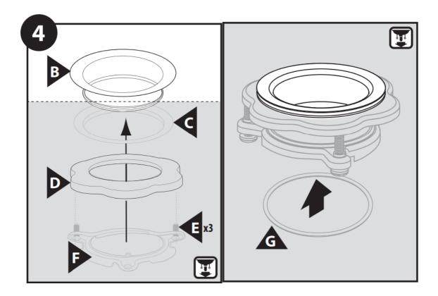
Re-assemble the fiber gasket (C), backup flange (D), upper mounting ring (F) and screws (E). From underneath the sink, place the fiber gasket (C), backup flange (D) and then the upper mounting ring (F) onto the flange in this order. Hold the fiber gasket (C), backup flange (D) and upper mounting ring (F) in place while aligning the snap ring (G).
