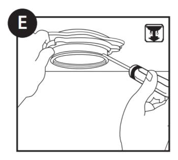
Inspect current mounting ring seals, your new diposal may be compatible with the existing mounting ring and could be reused. If the existing sink flange is to be reused, go to page 7, step 10. If unable to be used, remove the old sink flange from the sink. Clean the sink thoroughly.
