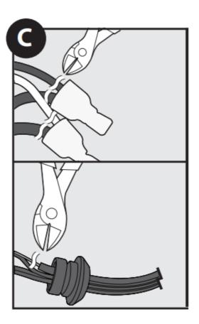
Cut white and black wires off close to the connectors. Pull cord out of housing. Cut green ground wire close to the cord strain relief.
