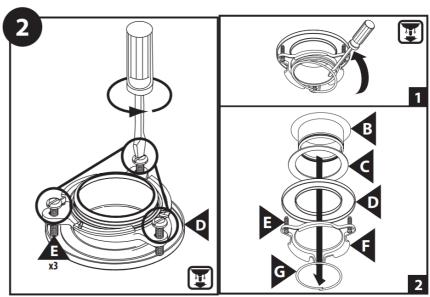
Remove disposal from packaging. Disassemble the mounting assembly from the disposal by turning the lower mount ring until it disengages from the ramps on the upper mounting ring.
