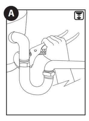
Unplug the disposal or if disposal is hardwired, turn off the electrical power at the circuit breaker or fuse box. Use a wrench to disconnect the drain line where it attaches to the disposal discharge tube.
