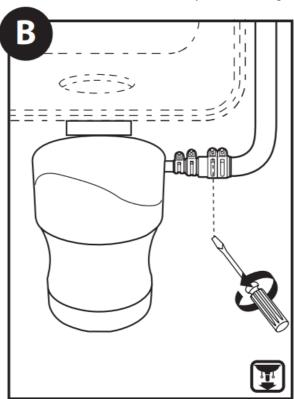
If a dishwasher is installed, make sure the dishwasher is not running. We recommend unplugging the dishwasher or turning off the electrical power at the circuit breaker or fuse box. Remove the dishwasher drain hose from the disposal.
