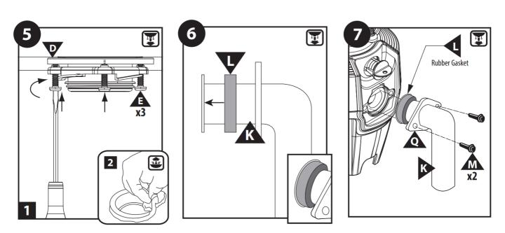
1. Tighten all three 1/2" Screws (E) evenly and firmly against the Backup Flange (D). DO NOT OVERTIGHTEN! Verify preassembled Gasket (L) is flush to flange on Elbow (K).
