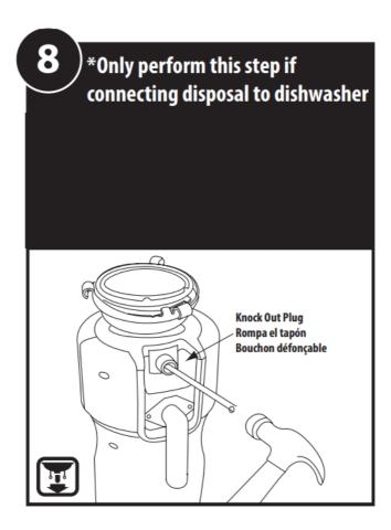
Using a blunt instrument (steel punch or wooden dowel), knock out the entire plug in the dishwasher inlet. Do not use a screwdriver or sharp instrument.
