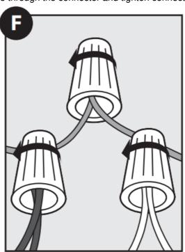
Connect internal disposal wire leads to coordinating wire lead from electrical source. Connect white to white, black to black or red, and green ground wire to the ground lead with wire nuts (not included).
