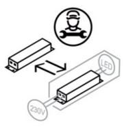
The separate control gear should be replaced by a qualified person.
