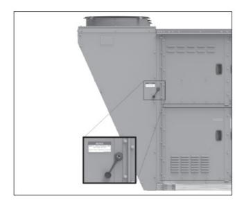
**Model Series "D", "H", "I", "O"** All Model Series "D", "H", "I", "O" units with the Modine Control System option include a unit mounted pLDPRO (Figure 2.3), which is a smaller version of the pGD1 interface. It features the same screen information and keypad functions but is unit mounted in a smaller package. Unit Mounted pLDPRO Interface
