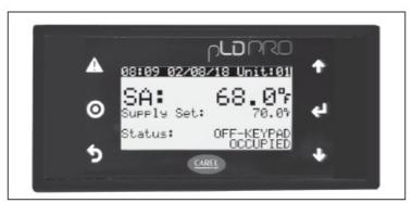
**Model Series "D", "H", "I", "O" (continued)** For remote access, the pGD1 can also be used, in addition to the unit mounted pLDPRO, as follows:
