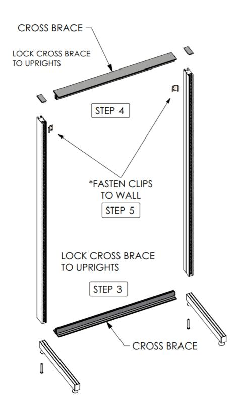
Disclaimer: Unit must be permanently secured and fastened to wall or other structure for stability.
