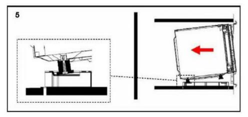
6. Adjust the position of the microwave with the position of the back legs into the holes on the buffer / support the back and most of the front legs into the holes on the buffer / support the front.
