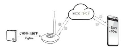
The ST3 Sensors use ZigBee 3.0 protocol to communicate with the Hub. Therefore, they are limited to a ZigBee range centered on the Hub (e.g., around the house). This range is affected by distance and obstacles such as walls, windows, water, radio interference, etc. In short, longer distances and more obstacles mean weaker signals.
