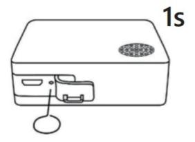
The Sensor is factory-paired with the Hub. After you have successfully added the Hub on the App, simply poke the pinhole with a pin for 1s then release and the Sensor will activate and paired automatically
