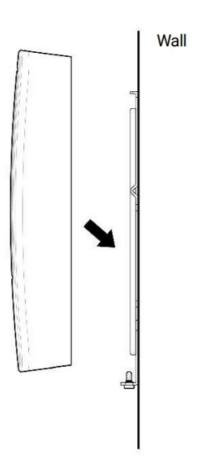
3. Assemble AE-MC with the bracket by rotating the product fixing screw.
