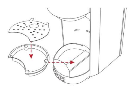
Attach the mesh plate to the mounting hole: Fit the tray into the recess on the bottom of the main unit.
