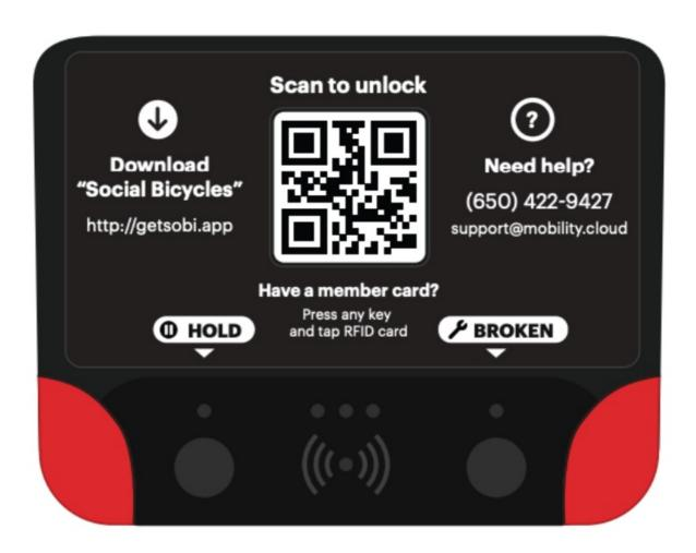
The two large circles are capacitive touch buttons intended for users to interact with the device. The left button puts a ride on hold, the right button reports issues with the bike, and all buttons wake up the module. The three small LEDs in the middle are use for status indication of the bicycle. The area in the middle is where the RFID antenna is located, and allows to start rental using RFID card.
